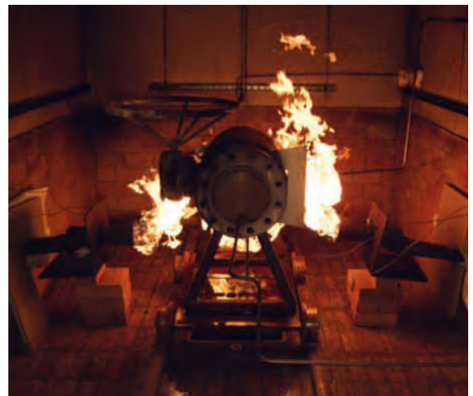
"Valves tested at independent fire test facility Scotland".
